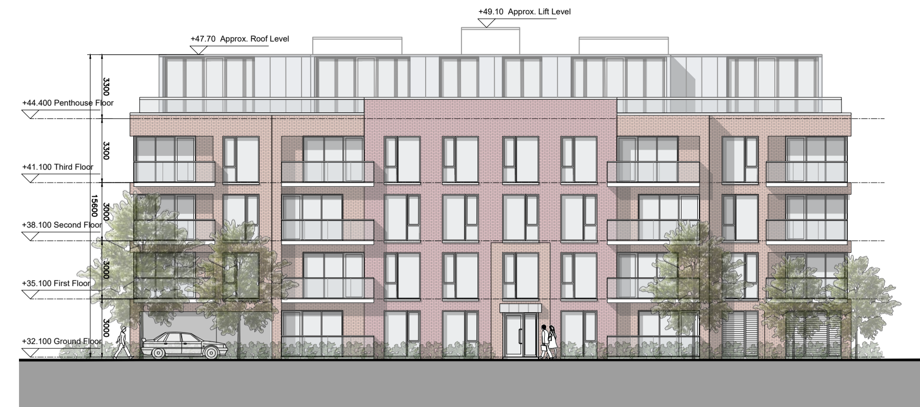
APARTMENT BLOCK B2 EAST ELEVATION (STREET ELEVATION)
