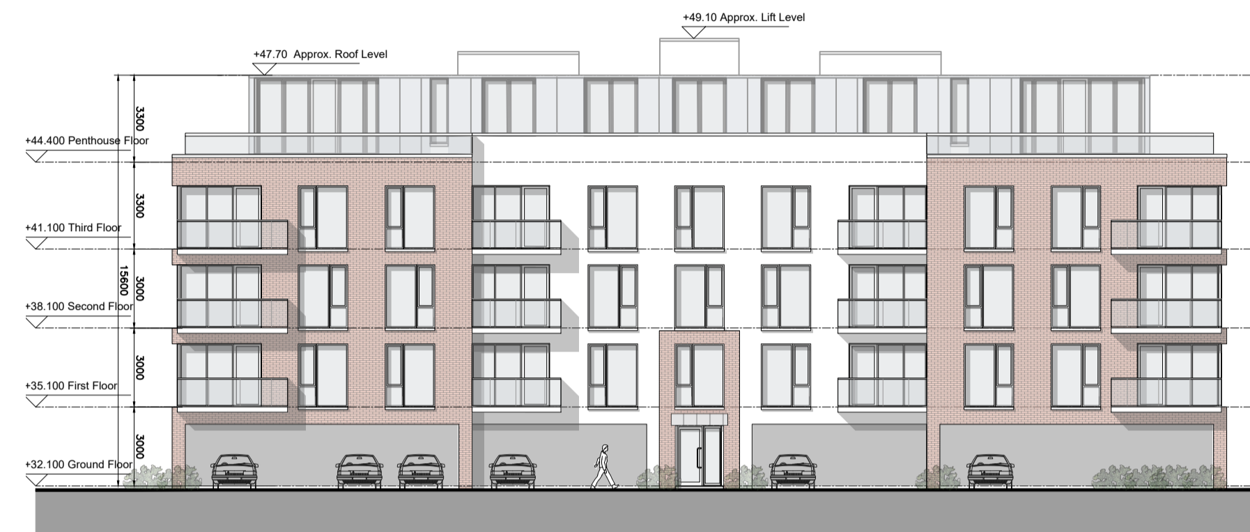
APARTMENT BLOCK B2 WEST ELEVATION (REAR)
